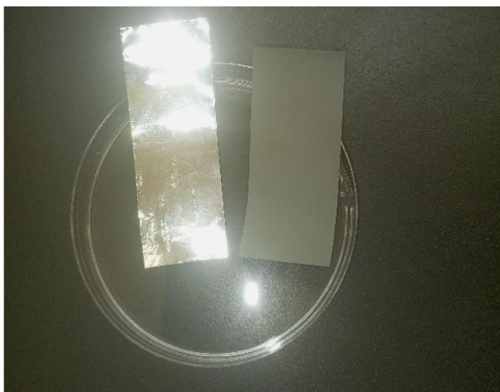
Figure 2: Anodized versus un-anodized aluminium foil (shiny)
