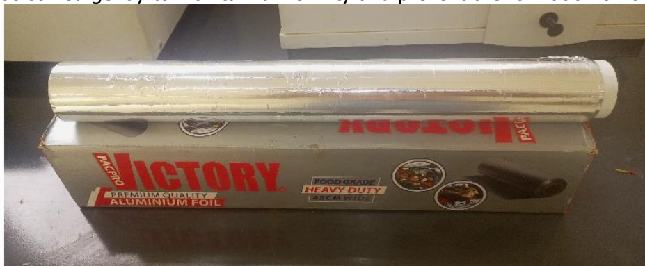
Figure 1: Commercial food grade aluminium foil served as the substrate
