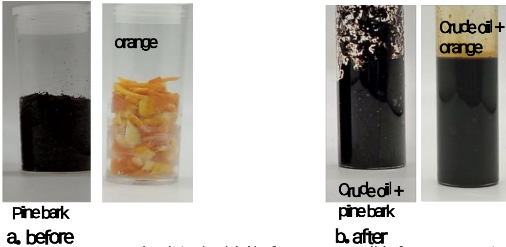
Figure 9 orange peel and pine bark (a) before treatment (b) after treatment in crude oil
