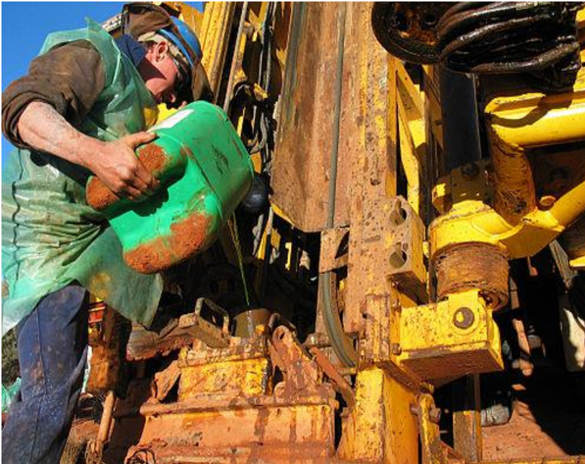
Physical manual handling of drilling fluids.
