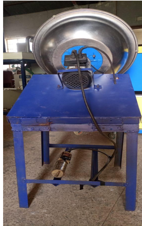
Fig 4.7 : The rear view of the drum with the motor, the drum mounting and frame of the machine
