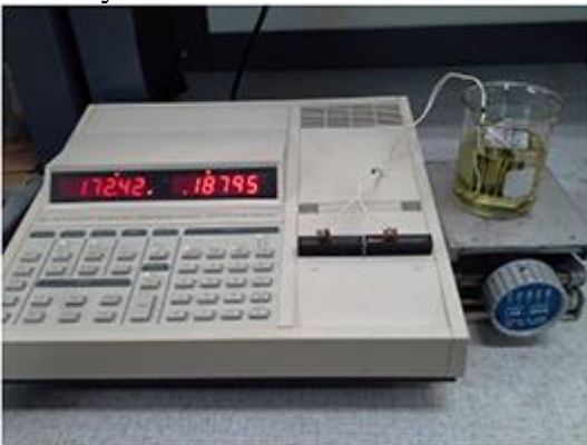
Figure 5. Capacitance measurement of the cell immersed in oil.
