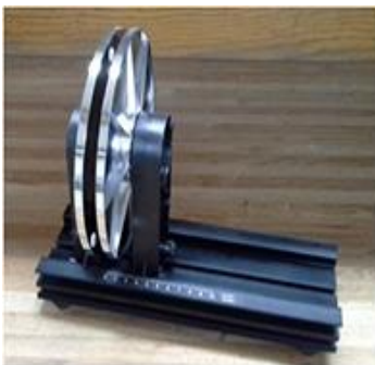
Figure 1. Parallel plate capacitor used for the basic experiment to measure dielectric constant Using a capacitance meter the capacitance C is measured and the dielectric constant k deduced using the well known relationship;
