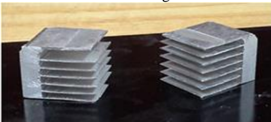
Figure 2. The heat sink cut into two parts.
