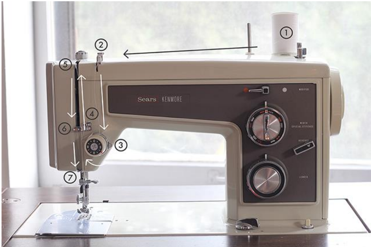
Fig 1.2 Order of Threading the Sewing Machine
